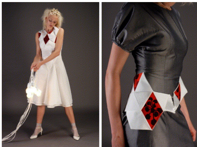
Fig. 10. An example of patterned polymer solar cells on a PET substrate incorporated into clothing by sewing through the polymer solar cell foil using an ordinary sewing machine. Connections between cells were made with copper wire that could also be sewn into the garment. The solar cells were incorporated into a dress and a belt. Design by Tine Hertz Reprinted from Sol. Energy Mater. Sol. Cells, 90, Krebs F.C.; Biancardo M.; Jensen B.W.; Spanggard H. & Alstrup J., Strategies for incorporation of polymer photovoltaics into garments and textiles, 1058-1067, Copyright (2006), with permission from Elsevier.
