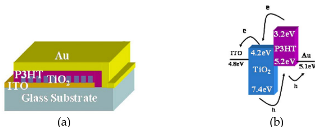
Fig. 12. (a) Schematic illustration of an inverted \text{TiO}_2 /P3HT hybrid solar cell manufactured by Kuo et al. using an AAO template for formation of parallel aligned \text{TiO}_2 nanopillars subsequently filled by P3HT; (b) Schematic illustration of the energy level diagram of the fabricated hybrid solar cell. Reprinted with permission from [Kuo et al., 2008]. Copyright [2008], American Institute of Physics.
