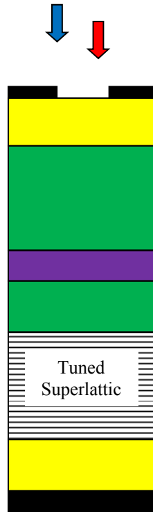
Fig. 8. Proposed cell structure: top cell p-n junction, tunnel junction (TJ) (purple) and p-i-n bottom cell with superlattice in the middle; P region (green), N region (yellow). Top cell is the window facing the sun (anti-reflected coating and surface texturing not shown).
